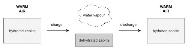
Figure 2: Sorption heat storage process for the zeolite 13X/water-configuration
