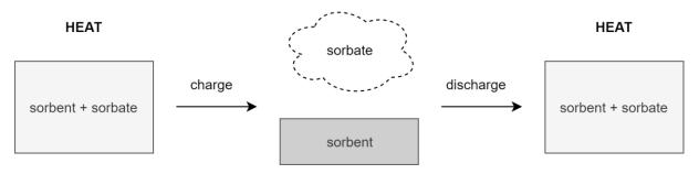
Figure 1: Sorption heat storage process
