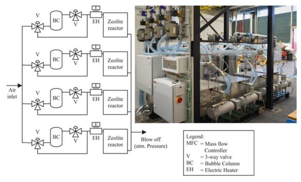
Figure 3: Simplified schematic overview (left) and picture of the of the experimental setup (right) [2].
