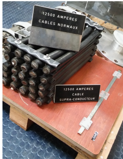
Figure 2: Size comparison between array of copper cables (left) and niobium-titanium superconducting cable (right), both rated to carry 12,500 amperes [6]
